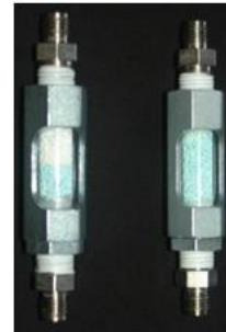
Figure 1. Color indicators used in sensor assembly; the indicator on the left capable of speciating COS and the indicator on the right without COS detection capability.
