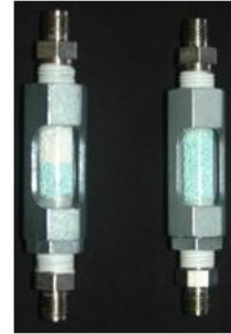
Figure 1. Color indicators used in sensor assembly; the indicator on the left capable of speciating COS and the indicator on the right without COS detection capability.
